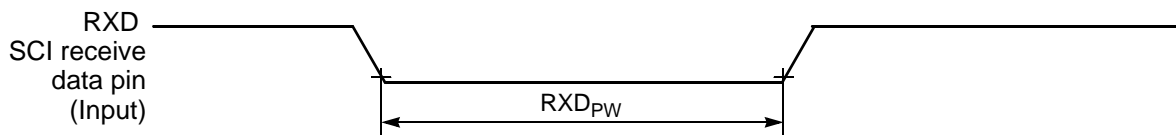
Figure 3-25 RXD Pulse Width
